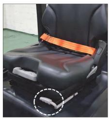
**NOTE:** The seat can only be correctly adjusted with the operator fully seated.
