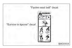
The "Survive in tipover" warning is located on the overhead guard. It shows the proper use of the operator restraint system.
