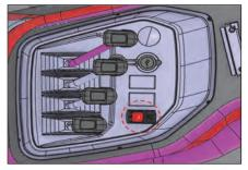
Push the front side of the parking brake switch to engage the brake and push the rear side to release it
