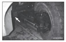
Inspect the suspension mounting bolts. Tighten suspension mounting bolts, if necessary, to 240  $\pm$  30 N·m (180  $\pm$  20 lb·ft).
