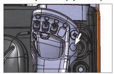
The auto clamp controller is at the rear side of the emergency switch. Pressing the auto clamp switch enables operation of the AUX2 knob. If not AUX2 operation signal is provided for 10 s after the trigger, the AUX2 will be locked. To reset the AUX2, press the auto clamp switch again. In addition, if no AUX2 operation signal is provided after key switch ON, the AUX2 will be locked up.
