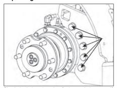
Check the bolt and washer for loosen bolt or nut; if any are worn or damaged, replace them. Check for any loose bolts and nuts, and tighten bolts and nuts if necessary(460±60 N·m or 340±44 lbf·ft)
