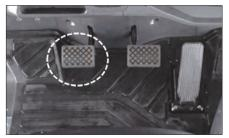
NOTE: The purpose of the inching pedal is to provide precise lift truck inching control at very slow travel speed and high engine rpm.
