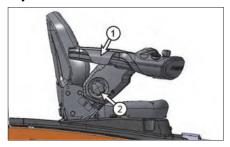
Using the two adjustment device, adjust the positions of the arm rests to a comfortable position.
