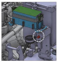
The main circuit breaker is located on the rear of the support for the hydraulic controls.
