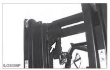
Inspect the part of the chain that is normally operated over the crosshead roller. When the chain bends over the roller, the movement of the parts against each other causes wears.
