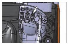
The side shift attachment controller is at the frontright side of the driver, and the side shift control lever is at the right as shown in the figure.
