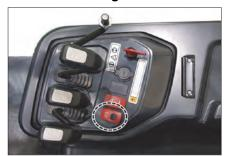
Push the front side of the parking brake switch to engage the brake.
