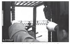
Inspect the carriage, forks or attachments for wear, damage and loose or missing bolts.
