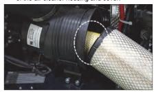
Remove the secondary element. Inspect the gasket between the air cleaner housing and the engine inlet. Replace the gasket if it is damaged.
