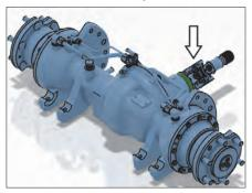
Check the bearings for wear and damage; if any are worn or damaged, replace them. Check for any loose bolts, and tighten bolts if necessary.
