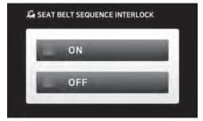
This safety function enables operation only when the seat is occupied and the safety belt is on.
