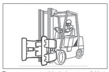
There are many special attachments available to replace the forks on a lift truck.
