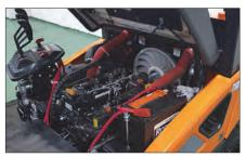
Inspect the engine compartment for oil, coolant and fuel leaks.
