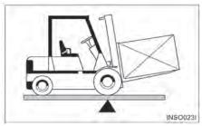
Counterbalanced lift truck design is based on the balance of two weights on opposite sides of a fulcrum (the front axle). The load on the forks must be balanced by the weight of the lift truck. The location of the center of gravity of both the truck and the load is also a factor. This basic principle is used for picking up a load. The ability of the lift truck to handle a load is discussed in terms of center of gravity and both forward and sideways stability.
