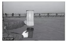
Insert a light inside the clean dry element and examine it. Discard the element if tears, rips or damage are found.
