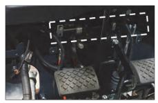
Lubricate three fittings for the inching and brake pedal control shaft.
