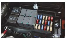
Check the fuses. Use a flashlight, if necessary.
