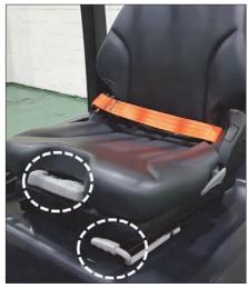
Check the operation of the seat adjuster rod. Make sure that the seat slides freely on its track.
