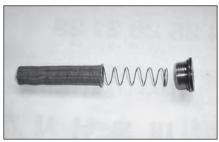
Wash the strainer assembly in clean, nonflammable solvent and dry it. Install the strainer assembly.
