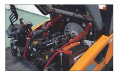
Observe the engine coolant level in the coolant recovery bottle. With the engine cold, maintain the level to the COLD mark. If the recovery bottle is empty, also fill the radiator at the top tank.
