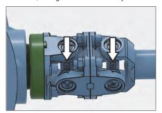
Inject a sufficient amount of grease into the grease nipples on the universal joint.
