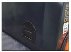
1. The engine compartment is accessible by pulling the latch.
