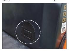
Push the lever down to raise the hood and seat assembly. Make certain the support cylinder will hold the hood open.
