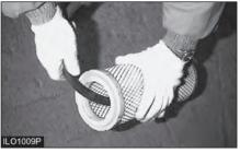
Direct water on the inside and outside of the element along the length of the pleats. Air dry it thoroughly and then examine it
