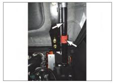
2. The hood and seat assembly is held up by a support cylinder. Make certain the air cylinder is operating properly and securely hold the hood up before doing anything in the engine compartment. To close the hood, push the red button on the cylinder and then pull the hood down.
