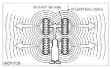
Do not approach a warm tire closer than the outside of the area represented by the shaded area in the above drawing. Dry nitrogen  $(N_2)$  gas is recommended for inflation of tires. If the tires were originally inflated with air, nitrogen is still preferred for adjusting the pressure. Nitrogen mixes properly with air.
