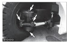
Lubricate the steer axle king pins, total of four fittings. Two on the right side and two on the left side.
