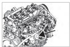
3. Remove and discard oil filter element.
