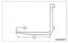
4. Check the difference in height of one fork tip to the other when mounted on the fork carrier. A difference in fork tip height can result in uneven support of the load and cause problems with entering loads.
