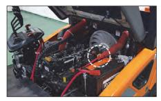
Measure the engine crankcase oil level with the dip stick. Maintain the oil level between the MAX. and MIN., (or FULL and ADD) notches on the dip stick.
