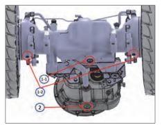
Remove drive axle drain plug (1-1), (1-2) and transmission drain plug (2). Allow the oil to drain into a suitable container. Clean the magnetic drain plug. Check O-ring seal and replace if necessary. Remove the spring and the strainer.
