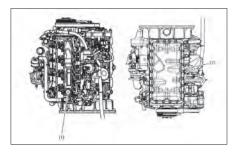
Using the oil filter cap (110910-00628), replace the oil filter (1).
