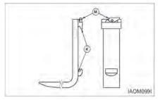
Check the fork mountings (K) for wear, crushing and other local deformation, which can cause excessive side to side wobble of the forks.
