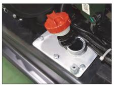
Remove the dip stick/filter cap. Maintain the oil level to the FULL mark on the dip stick/filter cap.
