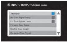
The vehicle digital signal can be checked (Alternator, RH turn signal lamp, LH turn signal lamp, forward gear signal, neutral gear signal, Backward gear signal)
