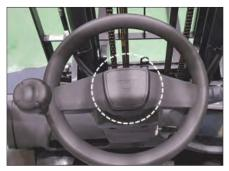
Press horn button, to determine if horn is operational.
