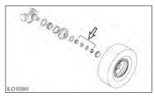
Remove the locknut, lock washer and flat washer.
