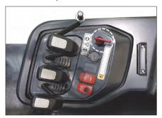
Lift trucks equipped with electrical disconnect switches; the engine will not start unless the disconnect switch is in the ON (closed) position.
