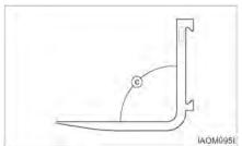
2. Check the angle between the upper face of the blade and the front face of the shank. The fork should be withdrawn from service if angle (C) exceeds 93 degrees or deviates by more than 3 degrees from an original angle other than 90 degrees, as may be found in some special application forks.
