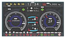
The engine oil pressure indicator light (17), will not come ON with the engine running, unless there is low or no oil pressure. Stop the engine immediately, if the light comes ON.
