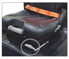
To position the seat, PUSH the lever away from the seat track and move the seat forward or backward to a comfortable position.
